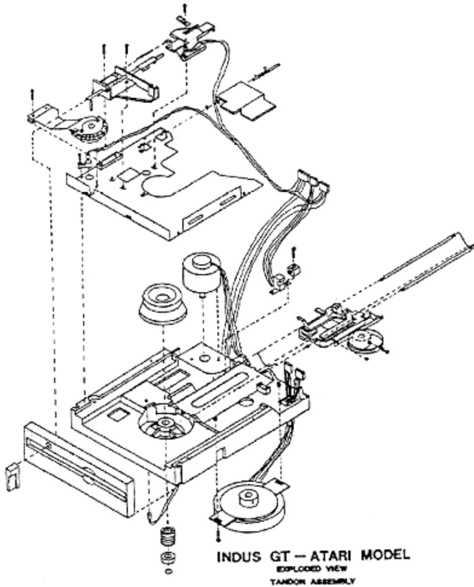
Take a close look at the ribbon cables. Older drives have bulky plastic connectors attaching the cables to the WART board. All of the later model drives have slim-line ribbon connectors. When you are ordering replacement parts be sure you specify which type of connector is needed.
