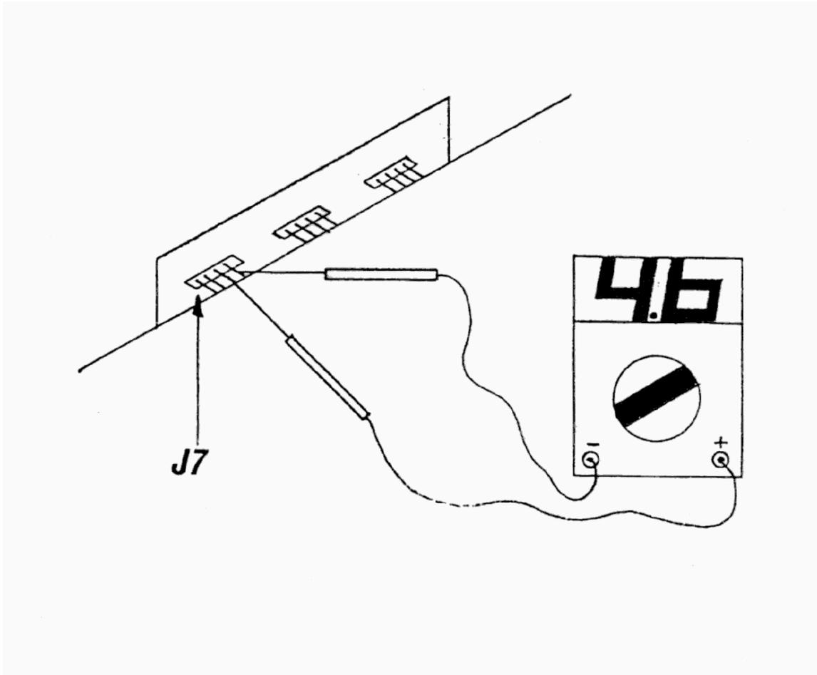
STEP 3. With the DVM set to the 20 VDC scale, observe that the voltage is between 4.4 VDC and 5.0 VDC.
