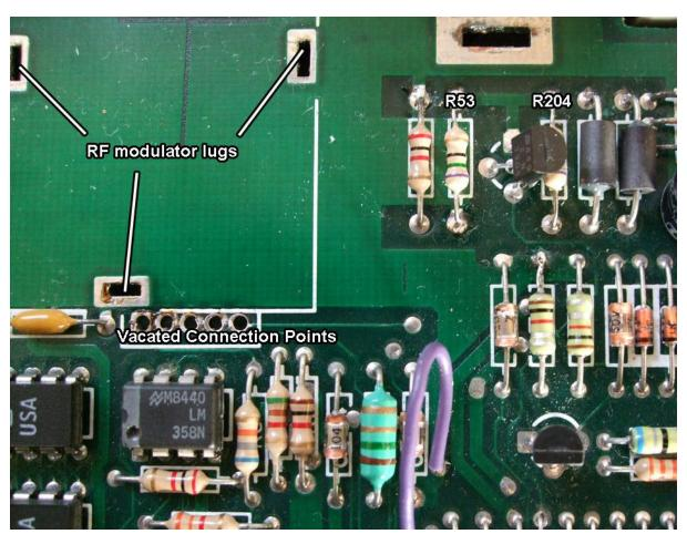
2. With the RF modulator removed, our next job is to replace the resistors R53 and R204 (on either side of the transistor Q3) with 750hm resistors as shown in the preceding illustration.
