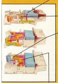
DISKETTE PICKER grasps the proper diskette and loads it into the drive accurately. The drive senses improper loading, and reclamps the diskette automatically.
